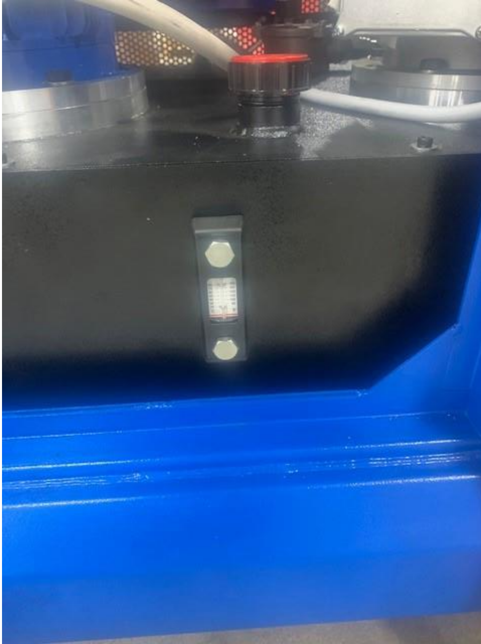
(Reservoir Sight Glass)
