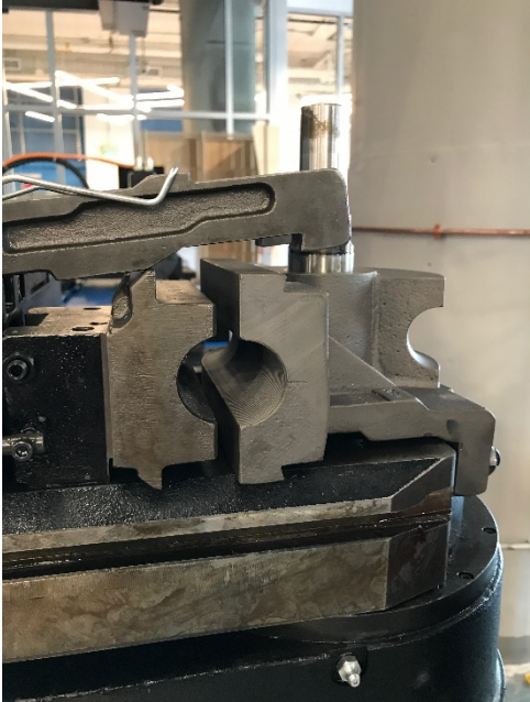
Slide clamp die cylinder forward and make sure the fingers are over the face of the former
