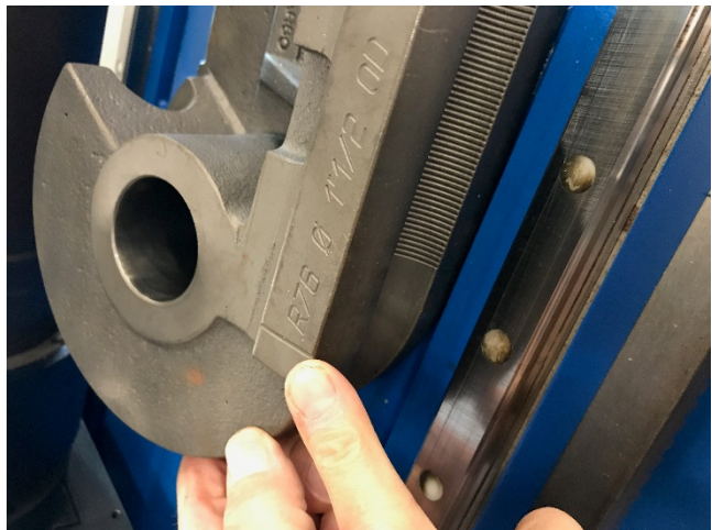
Bend die stamped "R76" to indicate 76mm center-line radius
