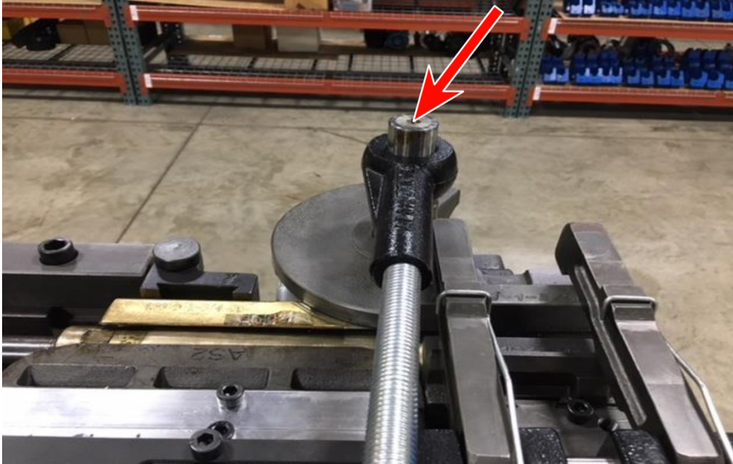
The reference point for all machine axes is the center of the tooling spindle
