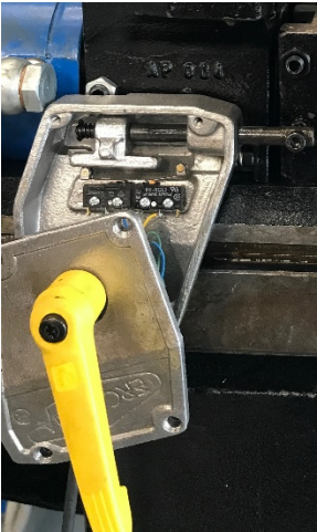
Clamp die limit switch box showing micro switches
