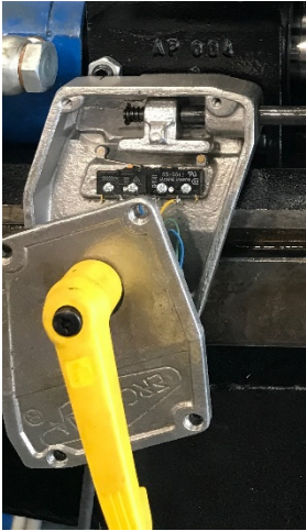
Only one switch can be engaged at a time for proper function
