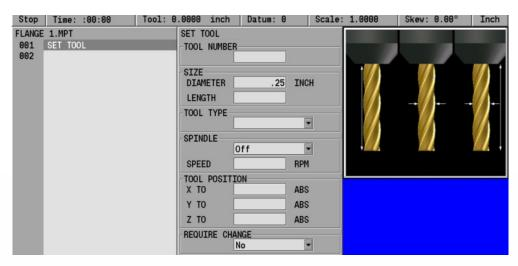
**STEP 1** – All programs begin with the tool. Parameters are entered in the middle column and are graphically supported in the right column for each field.
