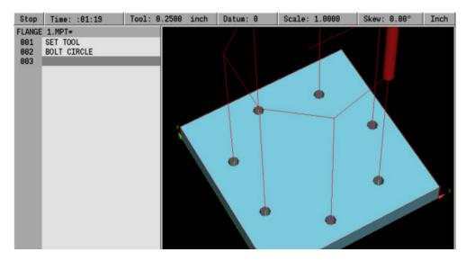
**STEP 3** – Once the circular bolt hole pattern data has been entered into the form press the USE hard key and a graphic of the program is displayed.
