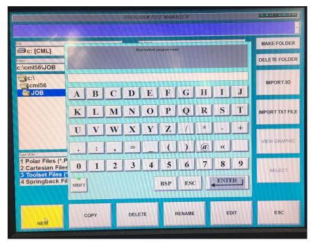
4. Begin entering data for your new toolset. The interface is highly graphic. Double click the field you wish to edit and a graphic will display showing you exactly what is required for that particular entry. Use the pop up keypad to enter the numeric values and press, "ENTER" when finished. (Several pop-up graphic screens are shown for reference)
