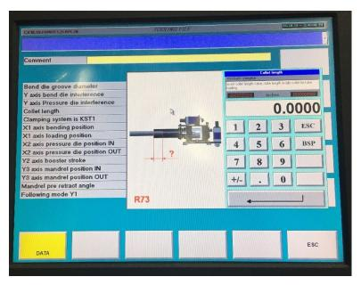
5. The first required field is "BEND DIE GROOVE DIAMETER". Enter the OUTSIDE DIAMETER of your material here. (Ex: 1-1/4" Pipe = 1.660 O.D.)
