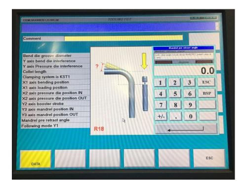
18. "FOLLOWING MODE Y1". The carriage or Y1 axis must always follow the material during the bending process. This must be set at 100 (100%) to ensure correct positioning of sequential bends.
