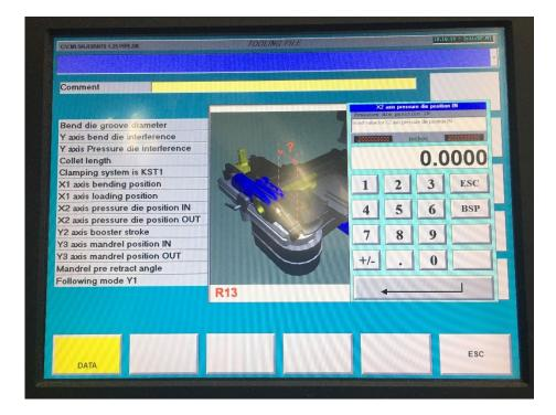
13. "X2 AXIS PRESSURE DIE POSITION OUT". This value is so the pressure die can be back and out of the way so the machine can position for the next sequential bend or come forward for the end of cycle. As a rule of thumb, the difference between the IN and the OUT position should be at least 5/8" (e.g., If the IN position is set at 6.00 then the out will be 6.625).
