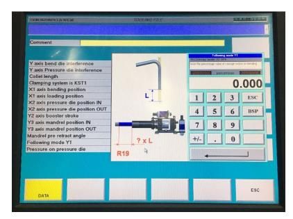
19. "PRESSURE ON PRESSURE DIE". The IN and OUT position of the X2 pressure die axis have already been set in the toolset file. This setting is meant to resist the tendency of the pressure die to be pushed out of position and exert additional forward pressure to maintain the set IN value. It is typically used when bending extremely heavy wall material or material near the capacity of the machine. For most bending, a setting of "NO" is used.
