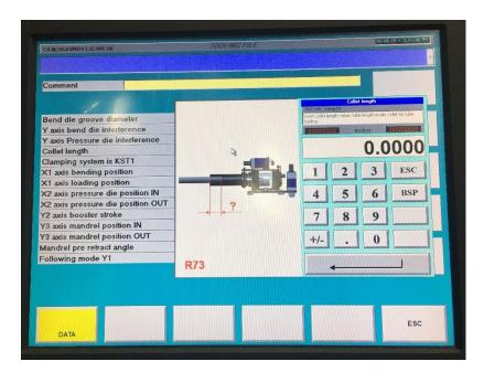
9. "CLAMPING SYSTEM is KST1". All ERCO series machines use FST or Finger Style Clamping systems and NOT the KST. The KST system is used on GB Series mandrel bending machines. A value of "NO" should be entered here.
