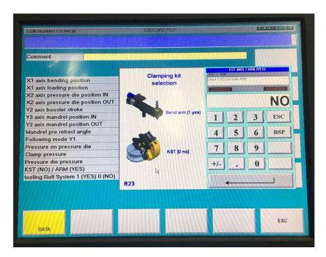
23. "TOOLING ROLL SYSTEM 1 (YES) 0 (NO)". Currently, all ERCO series mandrel bending machines only utilize a single stack of tooling for bending. This parameter is meant for future use and multi-stack tooling machines. The value input should be NO.
