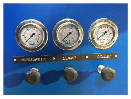
21. "PRESSURE DIE PRESSURE". This field is informational only. The pressure die pressure used for the material can be put here, as a reminder for the operator to change if needed. During the tooling set up, the pressure die pressure can be adjusted at the gages on the machine base. The set pressure should be input here on the toolset.
