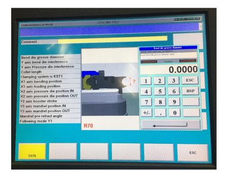
6. "Y AXIS BEND DIE INTERFERENCE". This number sets a mechanical limit on how close the carriage is able to come towards the center former. The wiper die and mounting bracket will limit the forward travel of the carriage. Also, note this value will affect the "last leg" length of your desired part. Machine must be able to position for the last bend to fully complete the automatic cycle.
