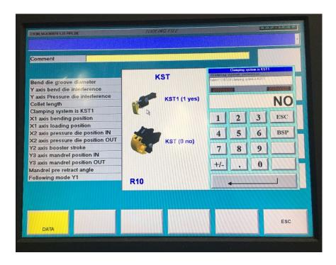
10. "X1 AXIS BENDING POSITION". On larger GB Series mandrel bending machines, the position of the bending head may be shifted to ease the loading and unloading of material. The ERCO series machines do NOT have this option so an entry here is not required. However, it is a good practice to put the centerline radius of the forming die in this field.
