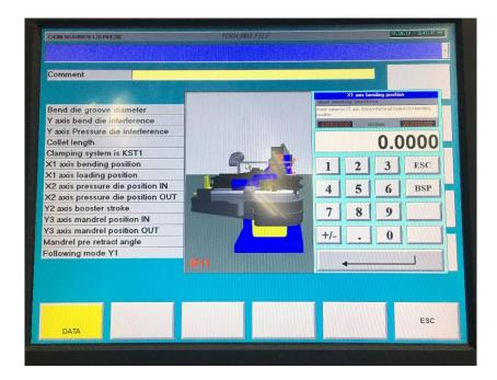
11. "X1 AXIS LOADING POSITION". On larger GB Series mandrel bending machines, the position of the bending head may be shifted to ease the loading and unloading of material. The ERCO series machines do NOT have this option so an entry here is not required. However, it is a good practice to put the centerline radius of the forming die in this field.
