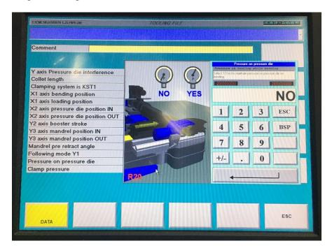
20. "CLAMP PRESSURE". This field is informational only. The clamping pressure used for the material can be put here, as a reminder for the operator to change if needed. During the tooling set up, the clamping pressure can be adjusted at the gages on the machine base. The set pressure should be input here on the toolset.
