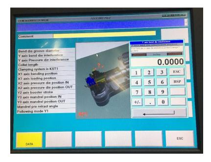
7. "Y AXIS PRESSURE DIE INTERFERENCE". The pressure die and mounting bracket will limit this position. All axis measurements are from the center of the tool spindle. The machine references that point as zero for ALL AXES.
