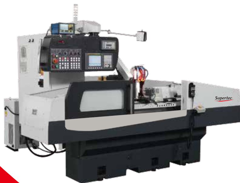
Angular Wheelhead ( GA Series ) Max. Grinding OD: 9"~19" Distance Between Centers: 20"~79"
