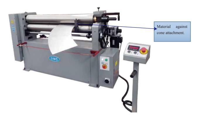
6. Push the up button switch or down button switch to adjust the bending roll position. Press the foot pedal to make the rolls turn.
