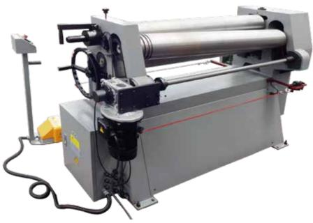
4.After the bending roll titling degree is set up correctly, please put the coupler back and connect properly, then tighten the set screw to lock the coupler.
