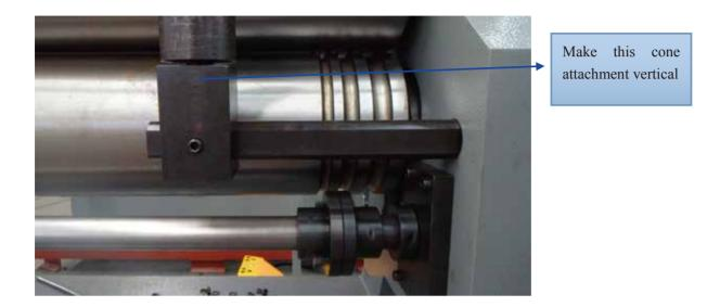
5. Put the sector material into the rolls, and crank the big hand-wheel to move the pinch roll up till barely touching the sector material, one side of the sector material will keep touching against the cone attachment while rolling it.
