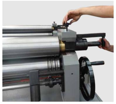
6.Rotate this handle counter clockwise 90 degrees, and hold and pull the top roller shaft to swing out the top roller, then remove the part out of the top roller. Then push the top roller back into the housing, and turn this handle clockwise 90 degrees, make sure the top roller sits correctly. Turn the black knob of the locking bolt to lock the top roller in position.
