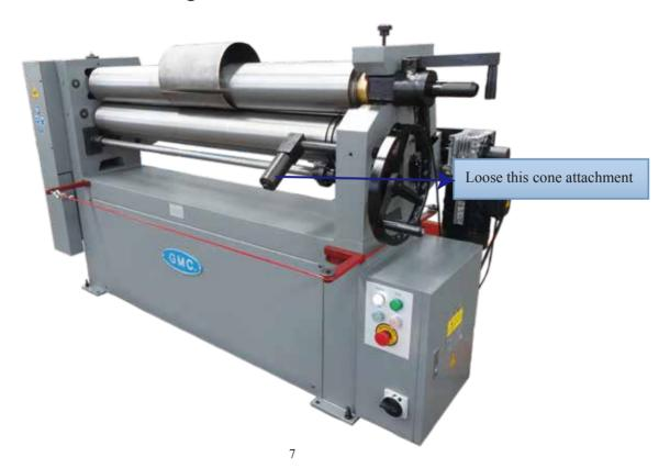
Press the foot pedal Loosen this locking bolt, get ready to swing out the top roller.
