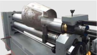
8. Loosen and turn the cone attachment down, and swing out the top roller to remove the cone part out.
