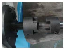
3. Push the up button switch to move right side of the bending roll up to make it tilt as shown in the picture below.
