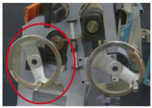
5. Press foot pedal forward and reverse to roll the material into the radius
