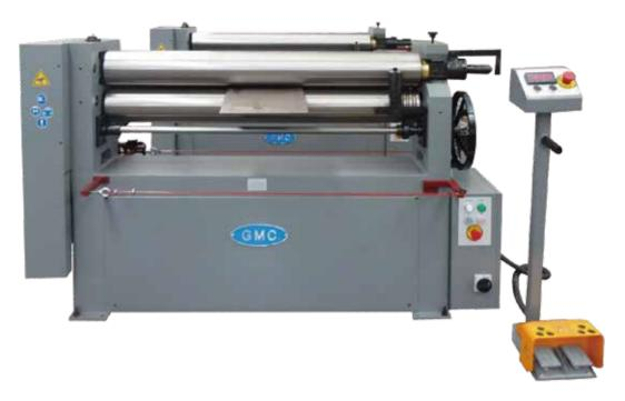
3. Push the up/down buttons to move the bending roll up/down for right position, and press foot pedal to roll the sheet metal material.
