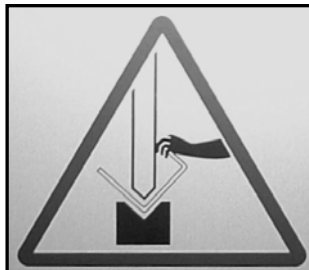
WHEN BENDING, HANDS MAY BE JAMMED BETWEEN TOP TOOL AND SHEET
