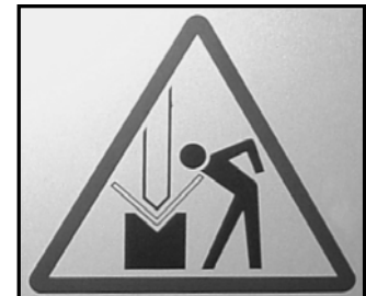
WHEN BENDING, SHEET MAY CRASH SOME PARTS OF BODY
