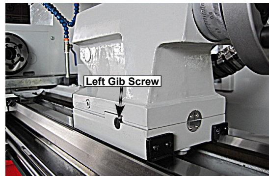
Figure 86. One of two tailstock gib screws.
