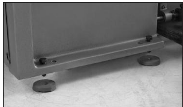
Figure 12. Leveling pads and screws.
