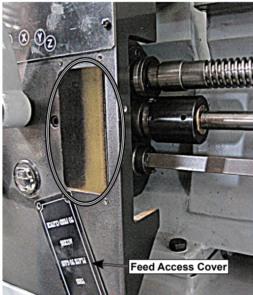
Figure 88. Feed access covers removed.
