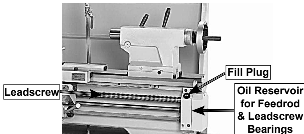
Figure 72. Leadscrew lubrication.
