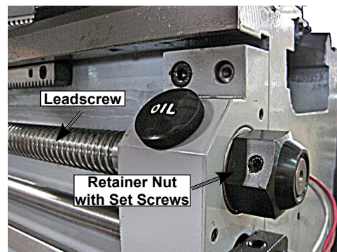
Figure 82. Leadscrew end play adjustment.
