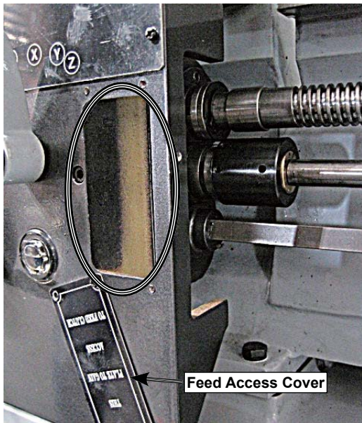
Figure 94. Feed access covers removed.
