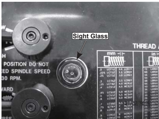
Figure 71. Location of the headstock oil sight glass.
