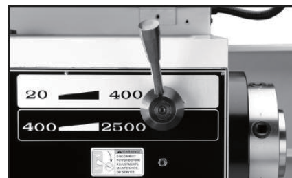
Figure 16. Headstock range lever.
