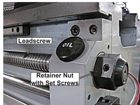
Figure 88. Leadscrew end play adjustment.
