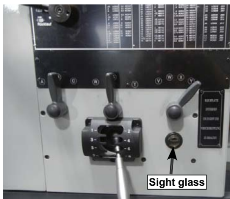
Figure 74. Gearbox sight glass location.
