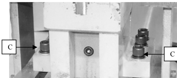
Six socket head cap screws (C) hold the die holder in place.
