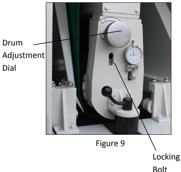
**Caution:** Abrasive belt must be a minimum .040 / 1 mm higher than the hold down rollers for proper feeding pressure. Failure to do so could cause possible improper feeding of the product and/or possible kick out.
