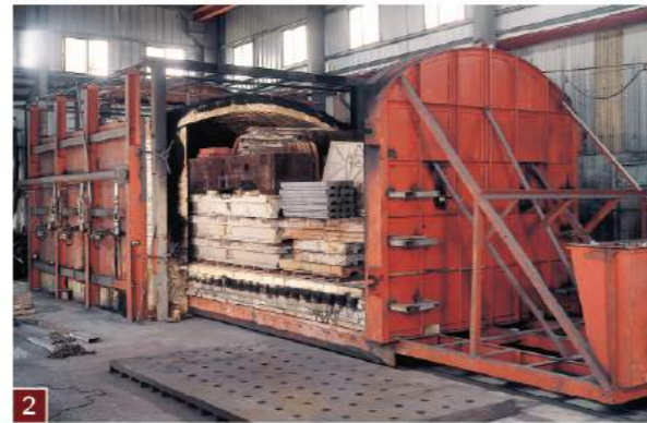
2 The exceptionally high-stiffness "MEEHANITE" casting undergoes an annealing process to eliminate internal stress prior to machining.
