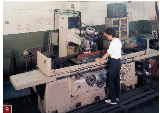
9 Precision grinding on dovetail-ways and the table bottom ensures a longitudinal guideline accuracy of 0.0004" over 50".
