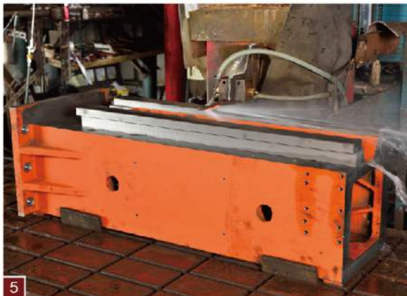
5 The Z-axis and all guideline surfaces, including the dove-tail ways on the table, are induction hardened to reach HRC 52 degrees.
