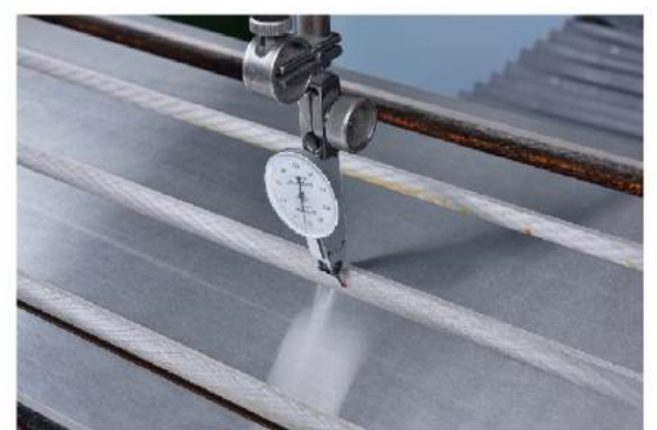
5 Parallelism of the T slot and X axis movement is also an inspection value. Normally per 40" the tolerated maximum number is 0.0008".
