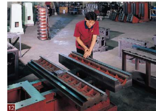
12 Before the saddle is loaded onto the machine base, the guideways of the saddle are fit to a table. The laminated gibs are then scraped on both sides to fit between the two components. This procedure on these mechanisms ensures and produces a lateral movement of less than 0.0004" per 40".
