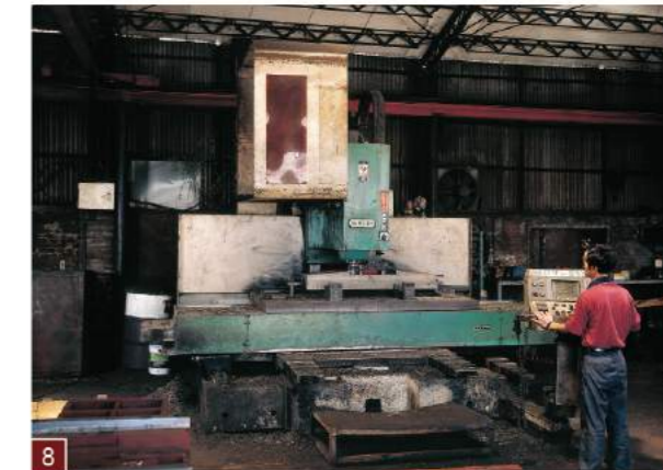
8 All contacting slideways on ACER saddles are laminated with Turcite-B. They are precision milled to maximize contact surfaces and allowing for time reducing hand-scraping procedure.
