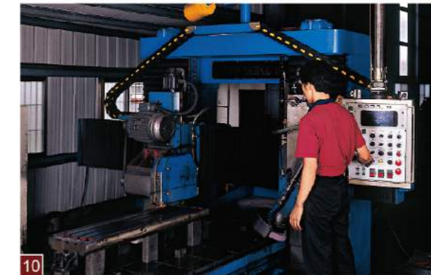
10 Using the precision ground dovetail-ways as the guideline, the table top is ground within 0.0005" over 50".
