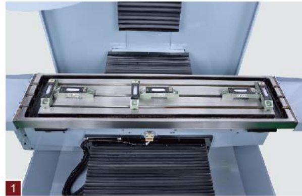
1 Flatness of the table is test on two directions. Both Z to X plane, and Y to X plane engineering levels should come within 0.0012" per 40".
