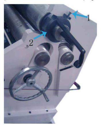
Put the steel plate through upper roller and front lower roller
