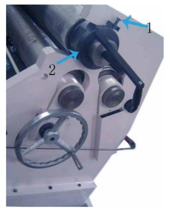
Then pull the upper roller to remove the formed part
