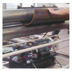
step on right foot pedal, steel plate moves backwards through the rolls; step on left foot pedal, steel plate moves forward
