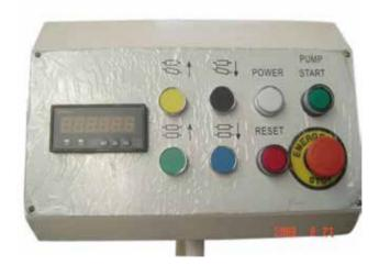
3)After power on, press the START button (on foot pedal) hydraulic pump runs, but if the upper roller isn't in the correct rolling place, all the actions of forward
