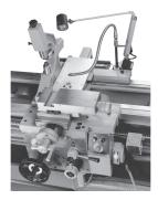
Carriage Carriage assembly features extended cross slide for accommodation of special tooling, tracer attachments, etc. The cross slide is constructed of high quality cast iron and incorporates externally adjustable nuts to provide for backlash elimination. The rugged, heavy duty taper attachment is capable of generating tapers of ± 10 degrees up to 15 3/4 inches long and is graduated in degrees for convenience of operation.
