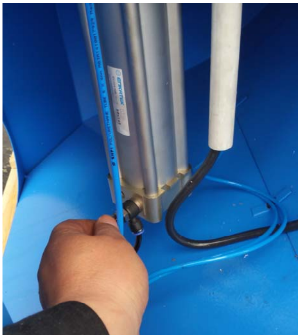
Adjusting the lowering speed
