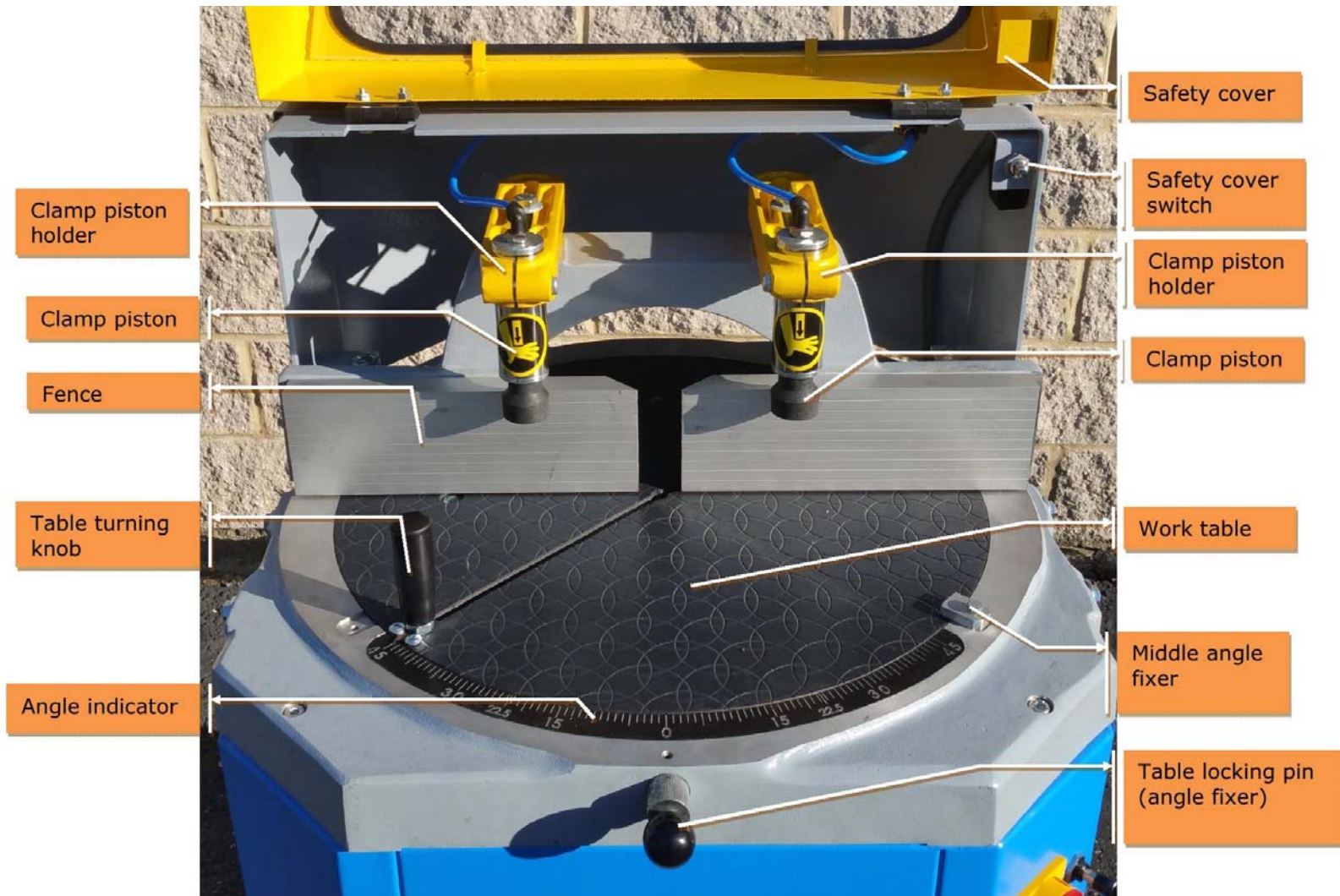
Description of the items on the cutting zone.
