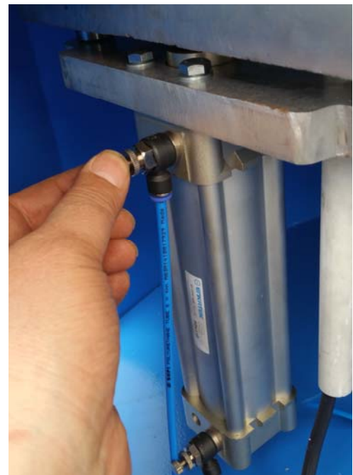
Adjusting the rising speed
