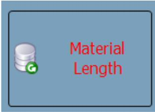
**Finished Material Length Button:** After finishing entering the command lines the length of the bent material has to be calculated. In the same time this button checks all the steps
