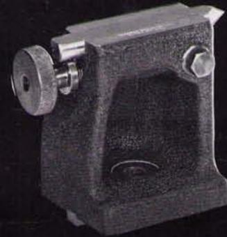
**T-4 TAILSTOCK** The hardened and ground spindle is screw fed and can be locked in any desired position with the hexagon clamp bolt. Removable
