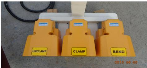
Or push the following circled black controller up to BEND position, the bending leaf will go up joggly and push the black controller down to release position, the bending leaf will go down joggly.
