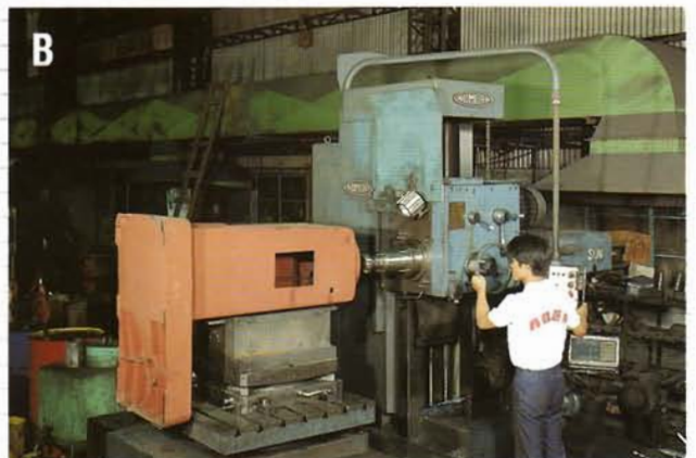
The foundations of accuracy (squareness, flatness & parallelism) are milled and machined extensively on planer-type contour milling or four-axis machining centers.
