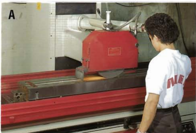
Precision grinding on top of the hardened table ( at HRC 52 degrees) to reach 0.0008" flatness over the table length.
