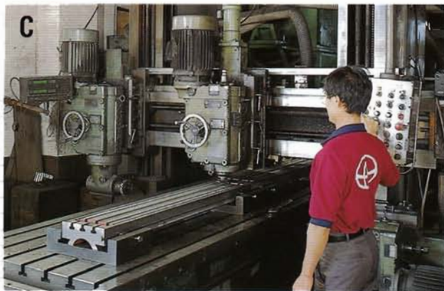
All tables are machined on bridge-type milling centers. The machining accuracy of the table will be within 0.0012" . The final grinding accuracy of the table can reach 0.0008" over 40" .
