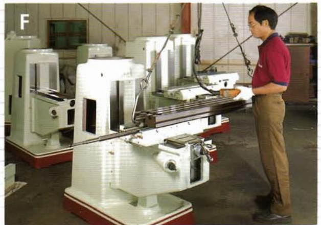
Once all saddles and lead screws are fit, the table is loaded onto the saddle. We can then finally adjust the table movement. A check and re-adjustment of the table is the final assembly procedure before inspection.
