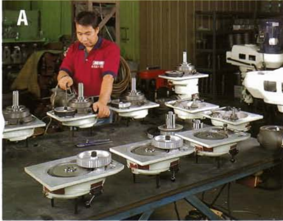
Carefully assembled lower housings are checked for braking mechanism and spline alignment. These two features reduce noise and vibration when the milling head is running.
