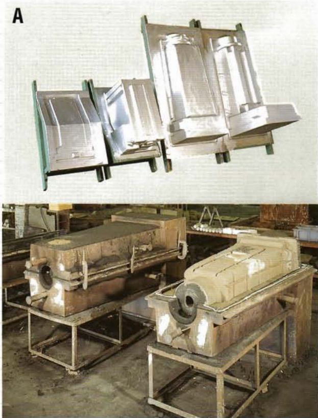
Ceramic-type mold-casting ensures rigid casting with ultimate conformance on casting surfaces.
