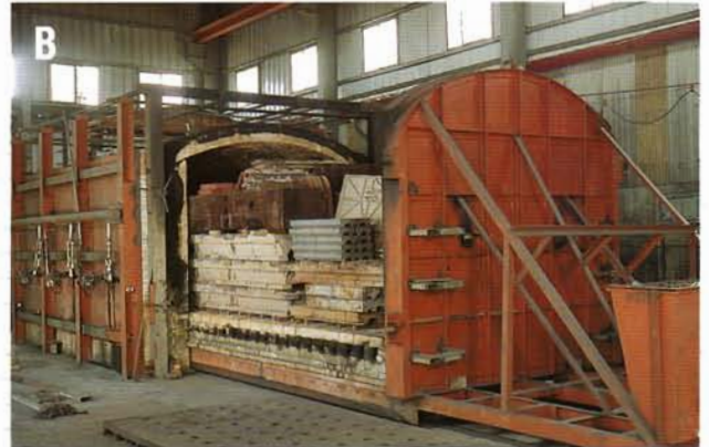
Exceptionally high stiffness "MEEHANITE" casting is treated with annealing process to eliminate internal stress prior to machining.
