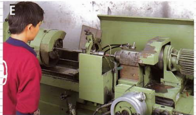
Every spindle is aligned and measured before final grinding. The high speed internal grinder is able to grind the spindle taper within 0.00008" of each other. This enables us to swap spindles to other machines and still keep the spindle run-out within 0.00015" .
