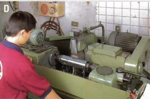
All quills are chrome plated and ground. The final cylindrical accuracy of the quill is within 0.0002" , and the bearing seat accuracy is within 0.00005" . This keeps the quill travel accuracy to within 0.0005" , and spindle run-out within 0.00015" . This prolongs the life of the spindle when operated properly.
