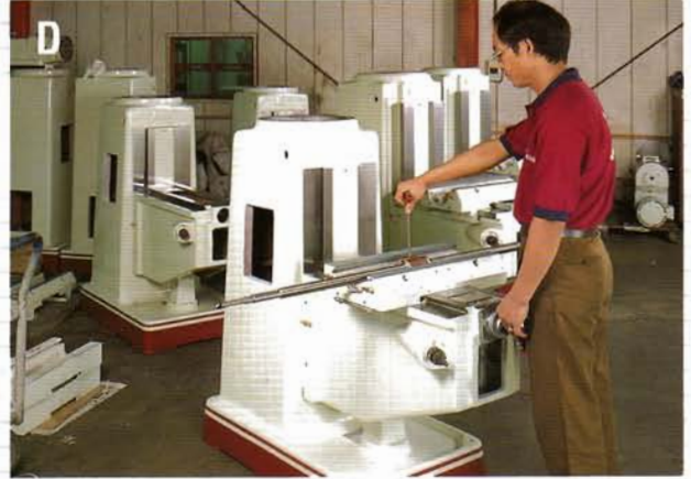
Technicians assemble the saddle onto the knee, and check for mis-alignment and irregularity. Once they are fit, the table can be assembled.
