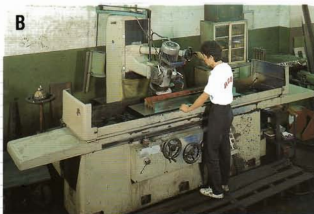
Precision grinding on dovetail ways and table bottom ensures a longitudinal guide line accuracy of 0.0004" over 50" .
