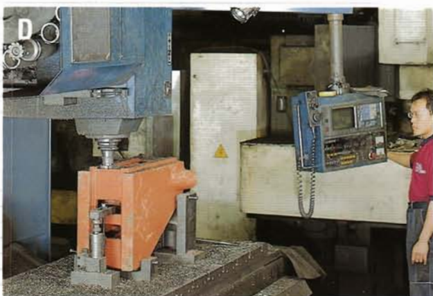
Every knee is put on a special fixture before machining. With this set-up, we can mill every knee perpendicularly within 0.002" of each other.
