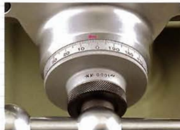
Backlash reading on dials. A: Max. 0.005" (longitudinal) B: Max. 0.005" (crosswise)
