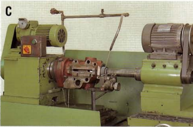
Precision grinding on spindle housing ensures the accuracy of the quill travel to within 0.0005" per 5".
