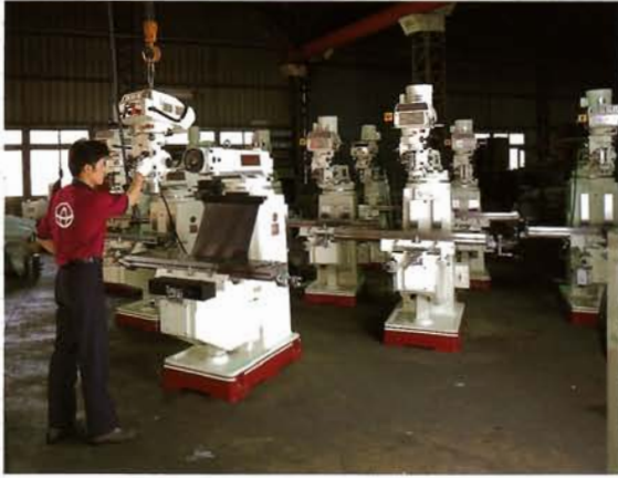
Adding the milling head is the final step before inspection. All ACER milling machines are produced to order, and shipped within the delivery time.
