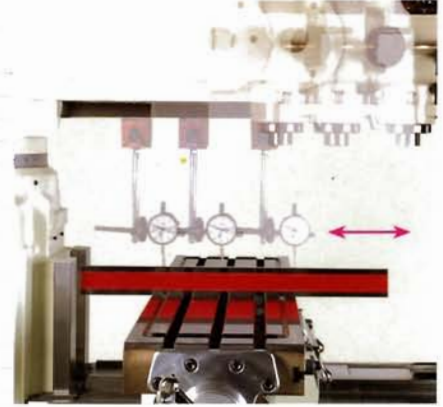
Ram slides parallel to table top. 0.0008/12"
