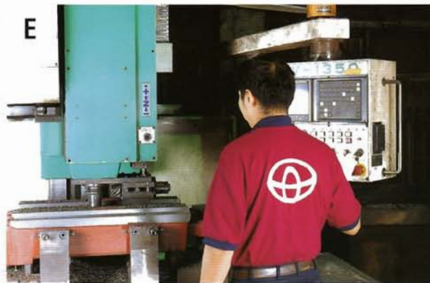
CNC machining centers are used to mill each ram. They are loaded onto fixtures and machined to the final accuracy of 0.001" per 20" .
