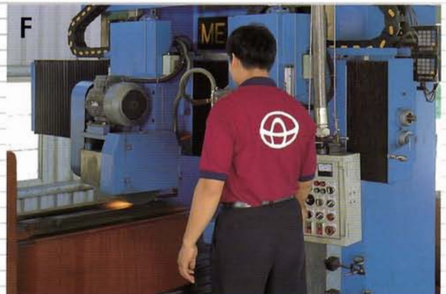
The special fixture on the double-column type surface grinder allows operator to grind machine column or knee in a very fast pace. It allows a higher than usual accuracy and parts will not deviate more than 0.0002" .
