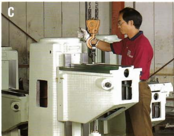
With extreme attention, the knee and column are assembled to reach inspection accuracy.
